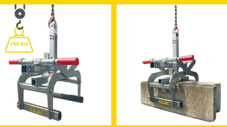
The AL750-UNI is the ideal stephandle for gripping and moving kerbs, steps and blocks etc. This universal galvanised clamp can lift up to as much as 750 kg / 1653 lbs. The AL750-UNI can automatically unlock and lock using the changeover automatic.
