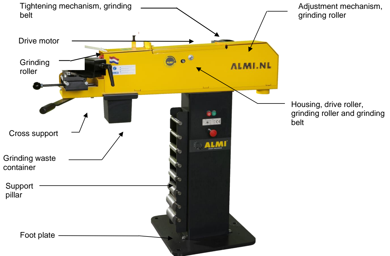
Figure 4.2-1: Construction of the machine
