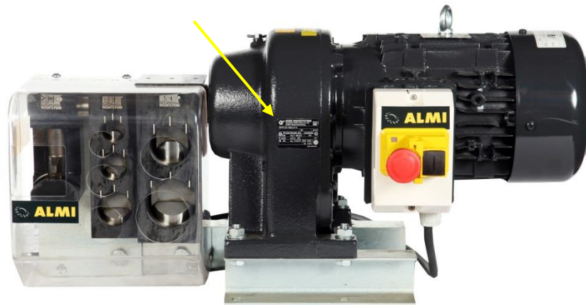
Figure 2.3-2: Location of the type plate
