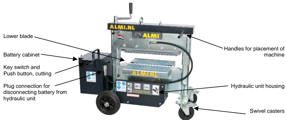
Figure 4.2-1: Construction of the machine
