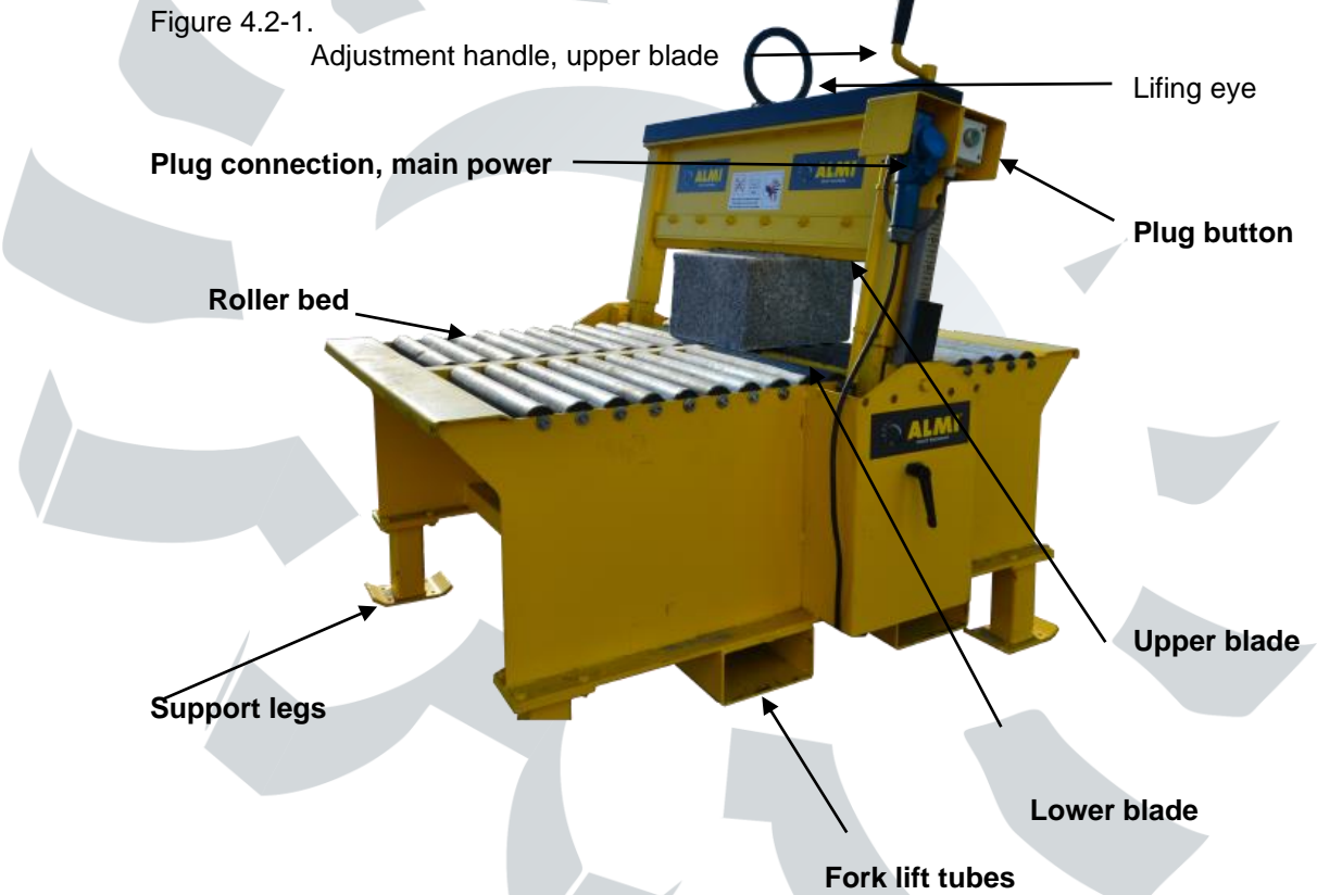
Figure 4.2-1: Construction of the machine
